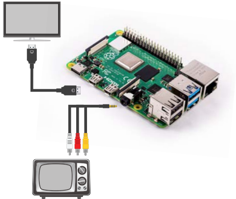
Figure 3. Connecting a display to the Raspberry Pi
