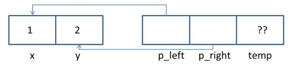
Now the function has access to the memory that backs those two variables, so when it performs its switch, it writes into the memory of variables x and y. First, it copies the value pointed to by p\_left into the temp variable, and then it copies the value pointed to by p\_right into p\_left:
