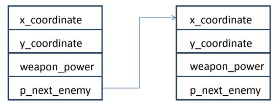
Here, we have one EnemySpaceShip structure that has a link of some sort to the next structure. What might that link be? A pointer! Each space ship has a pointer to the next space ship:
