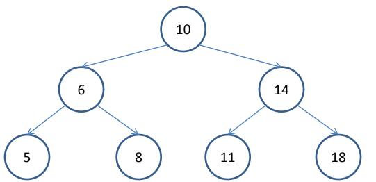
If we remove 10 from the tree, the remove function will immediately hit the "found" case. It will find that there are both left and right sub-trees, so it will find the node with the maximum value in the sub-tree headed by 6. That node is 8. It will then link 8's left sub-tree to point to the new sub-tree headed by 6, but that does not contain 8.
