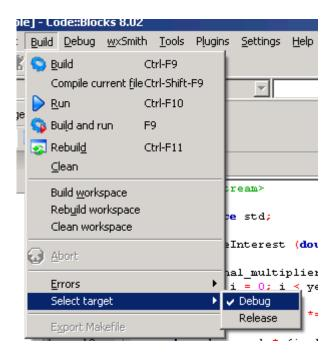
This will make sure that you build your program using the debugging symbols that you set up for the "Debug" target.
