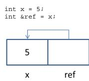
Here, the actual memory of the ref variable holds a pointer to the memory of the x variable. The compiler knows that when you write plain old ref, you want the actual value pointed to. In a sense, references are pointers with a reversed "default" behavior for what happens you write the name of the variable.
