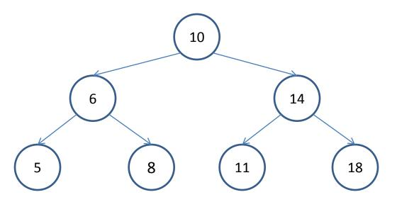
Notice that in this tree, left child of each element is a smaller value than the element, and right child of each element is larger than the element. Node 10 is the parent of the entire tree. Its child nodes, 6 and 14, are the parents of their own, smaller, trees. These smaller trees are called **sub-trees**.
