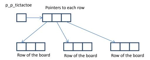
The first pointer points to a collection of pointers, each of which points to one row of the board. Here's the code that we need to allocate this kind of data structure:
