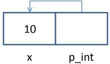
As I hope you have seen, using box-and-arrows diagrams can make it easy to follow what happens when you work with pointers. Whenever you get confused about what is happening, draw out the initial state of the memory, and then walk line-by-line through the program, showing how the memory changes. When a pointer changes where it points, draw a new line; when a variable changes a value, update its value. By doing this, you will be able to see and understand even complex systems.
