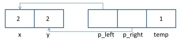
Notice that the memory that holds the  $_{\rm Y}$  variable has been modified this time. Finally, the value in temp
