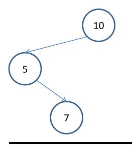
Since 10 already had a pointer to the node containing 5, re-linking the left child of 10 to the tree with parent 5 isn't strictly necessary, but it removes an extra conditional check from the code to check whether the sub-tree is empty.
