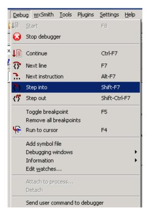
The Step Into command goes *into* the function that is about to be called on the current line, unlike Next, which will merely execute the whole function and show you the result, as we saw with the cin function. You use Step Into when you need to debug inside of a function, as we do here.
