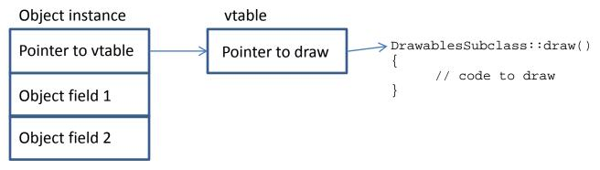
Because the object carries around its own table of methods to use, the compiler can change the addresses in the table when compiling different classes in order provide a specific implementation of a virtual method. Of course you don't do this yourself—the compiler does it for you. The code that uses the table just has to know exactly the right index to use for each virtual method to find it in the table.
