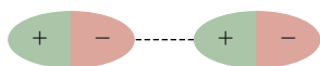
FIGURE 4.3 A dipole–dipole attractive force. Two molecules of a polar substance are oriented so that the positively polarized region of one and the negatively polarized region of the other attract each other.
